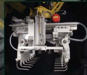
Finger gripper equipped with automatic bag width adjustment system
