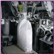
The upper transport unit jaws grab the top of the bag and move it toward the closing system in synchronization with the outfeed conveyor.
