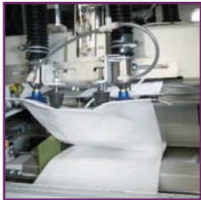
The pick-up unit lifts an empty bag from the magazine and releases it onto the feed conveyor.
