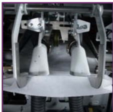
Spacers enter into the bag, side clamps pinch the bag, then the transfer arm swivels to place it onto the spout.
